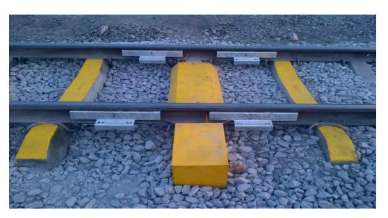
The RW-WM comprises a trade accuracy retrofit technology which is built onto the existing rail tracks, with no rail cutting or sleeper replacement, thus making for rapid installation.
