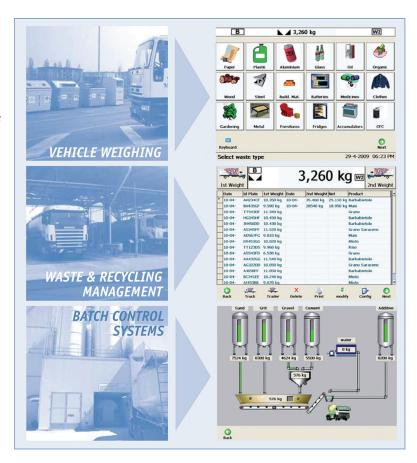
BATCH CONTROL software is available for weighing systems to control and manage weighing cycles, recipe formulae, silos, products, statistics, fast and slow filling and emptying plus automatic in-flight correction.
