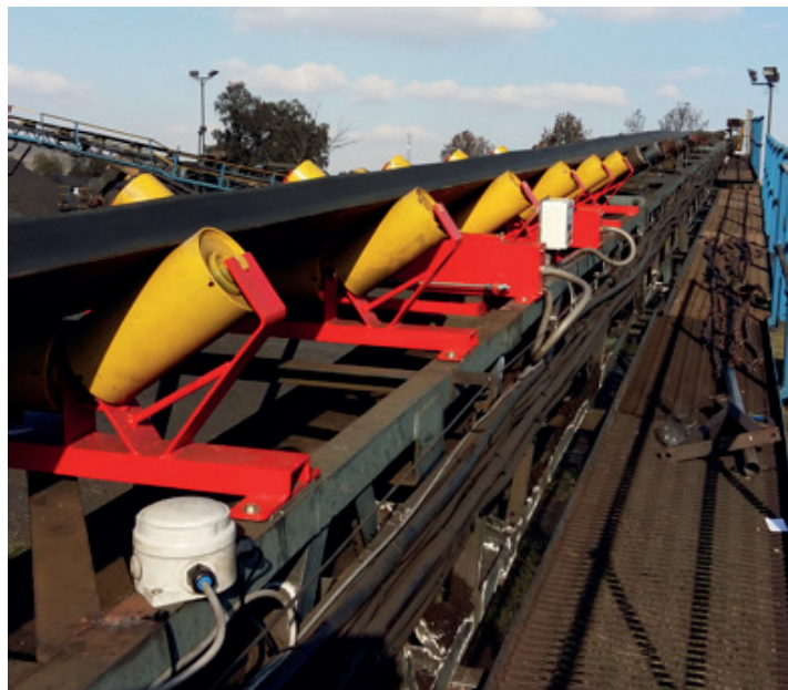
Typical in-situ belt scale on product feed application.
